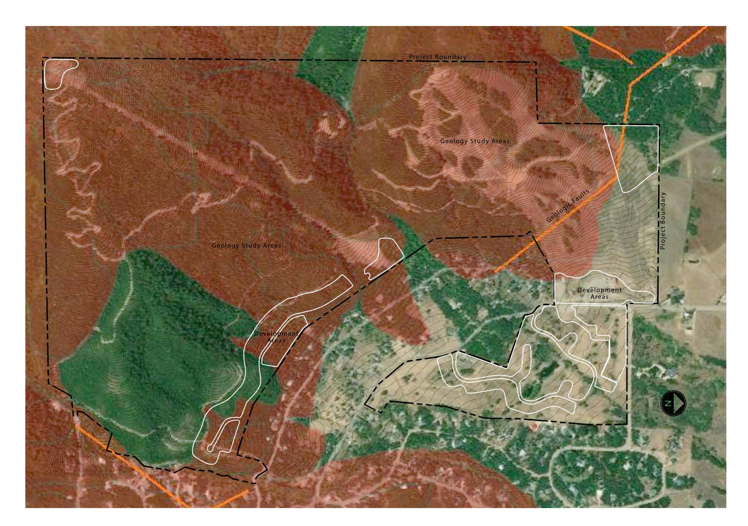
The Geology Study Area and Fault Exhibit here identifies surficial geologic conditions at the Project and identifies potential risk from geologic hazards.
