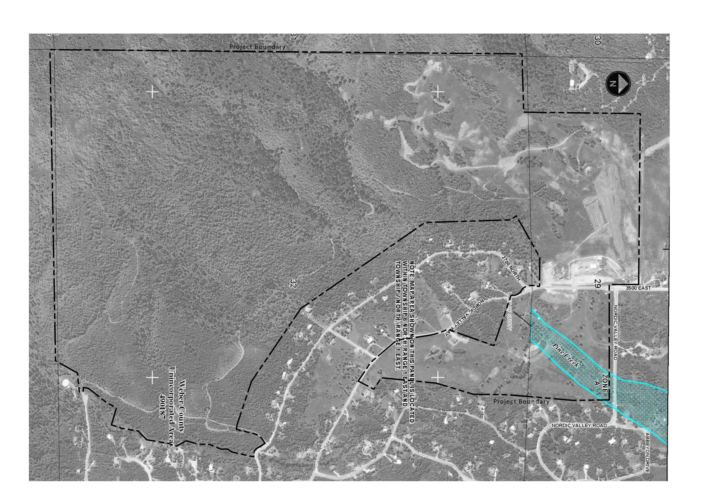
The FEMA Flood Insurance Rate Maps for Weber County illustrate that there is one flood area mapped within the Nordic Valley project boundaries. This Zone is identified as Zone A. As defined, Zone A base flood elevations are undetermined. All development within this Zone A area will provide further detail for floodway avoidance at the time of building permit or site plan applications.
